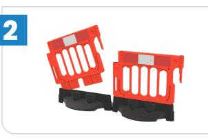
Line the second barrier up with the first. Tilt at an angle. Allow the prong on the end to slot into the hole on the barrier on the ground. Once the connection is made, slot the bottom of the barrier into the base.
